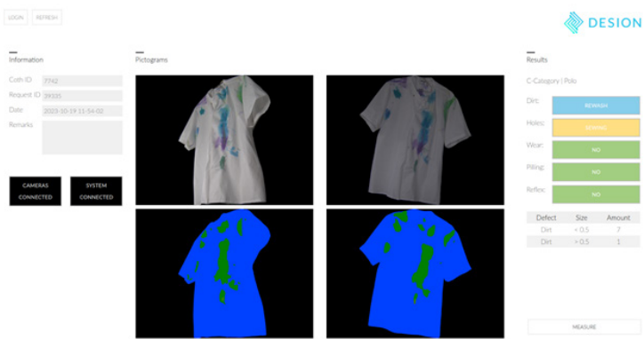
NIPS defects detection
